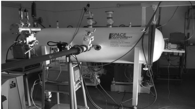
Fig. 2 Near-Earth space conditions vacuum simulating chamber.
